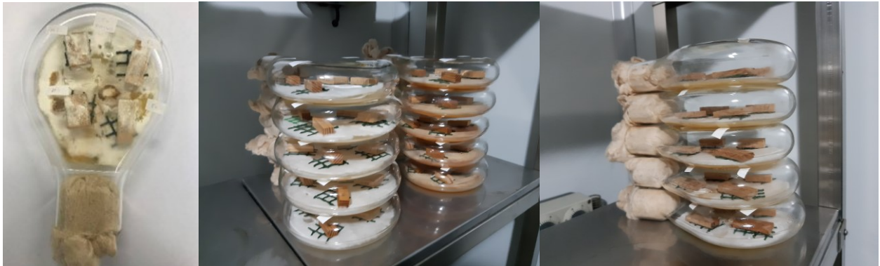
Figure 2. Rot fungi – 3 fungi – Maritime pine control, with 6 weeks of exposure and 10 replicated (with and without washout test) – Result – Very Susceptible.
