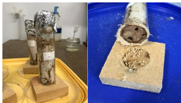
Figure 4. Reticulitermes Grassei – EN118 e EN118 + wash test (EN84) – Maritime pine control (n=3) – 8 weeks of exposure – 8 replicates – Result – Very Susceptible.
