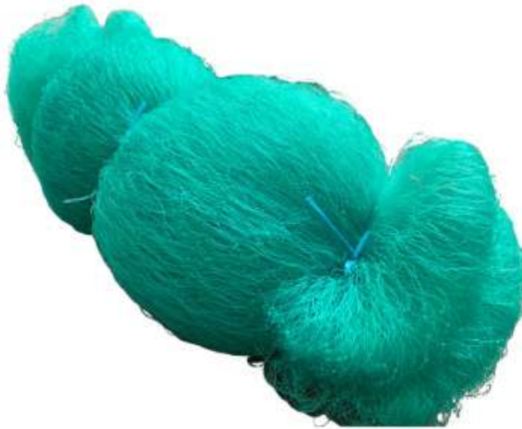
Figure 4- Fishing gillnet made of PBSAT monofilament used in this study.
