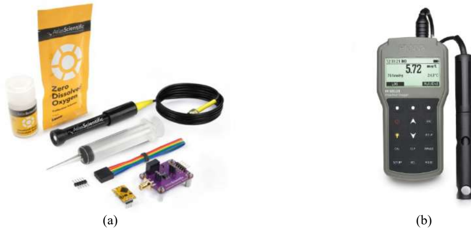
Figure 7-Sensores used to measure the dissolved oxygen present in seawater during the biodegradability tests: (a) EZO-DO AtlasScientific; (b) HI98193-HANNA INSTRUMENTS.
