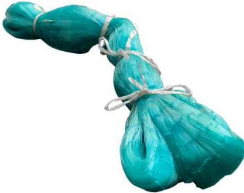
Figure 5- Fishing gillnet made of polyamide monofilament used in this study.
