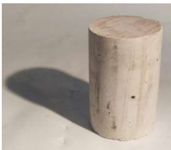
Figure 36 – Marble residue specimen (after unmolding)
