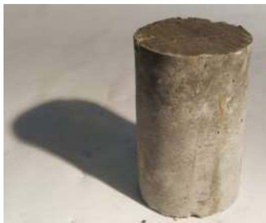
Figure 41 – Granite residue specimen (after unmolding)
