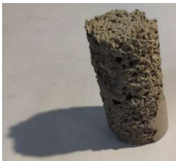
Figure 18 – BAGLASS glass residue specimen (after unmolding)
