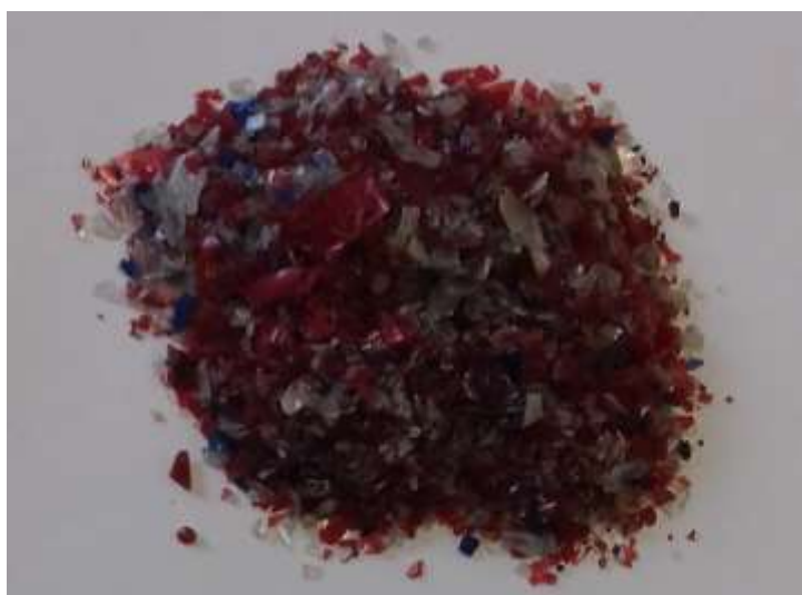
Figure 24 - Photography of plastic residue after milling.
