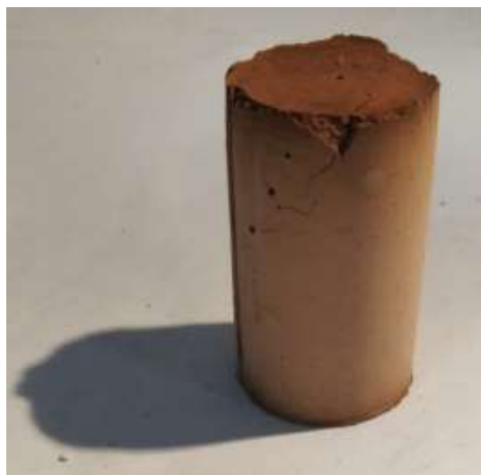
Figure 23 – Ceramic residue specimen (after unmolding)
