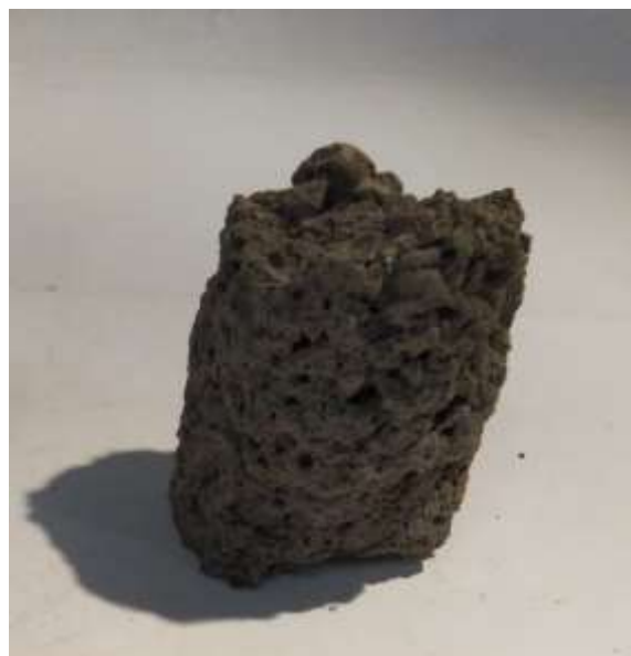
Figure 10 - LIPOR slag specimen (after unmolding)
