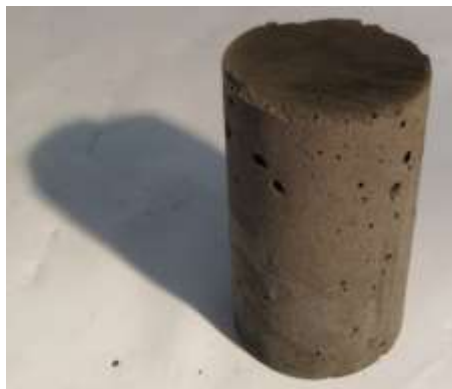
Figure 31 – Fly ash residue specimen (after unmolding)
