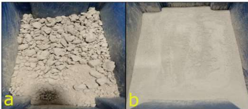
Figure 32 - Marble residue before (a) and after (b) sieving
