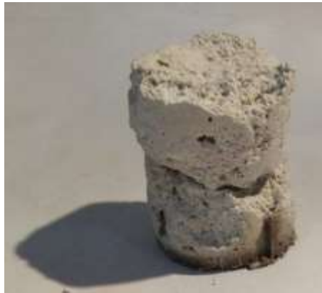
Figure 14 – Lens glass residue specimen (after unmolding)
