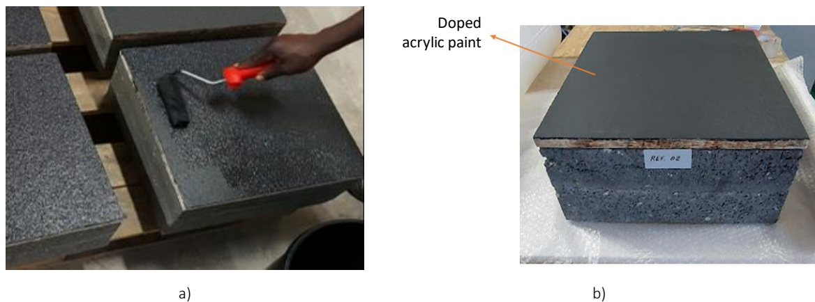
Figure 27: a) Doped acrylic paint application; b) Finished panel – Reference 2.
