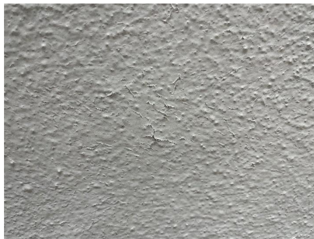
Figure 33: Surface cracking (primer) after ageing – Reference 3
