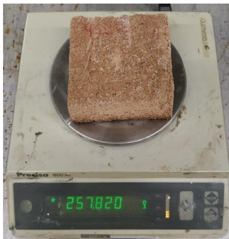
Figure 6: Weighing samples for water content determination.
