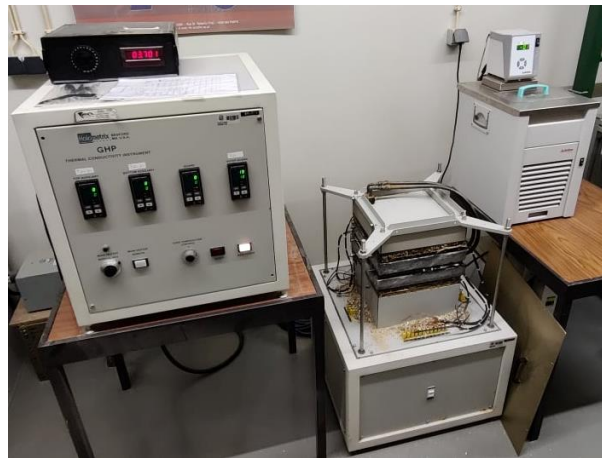
Figure 2: Holometrix GHP-300 – Guarded Hot Plate equipment.
