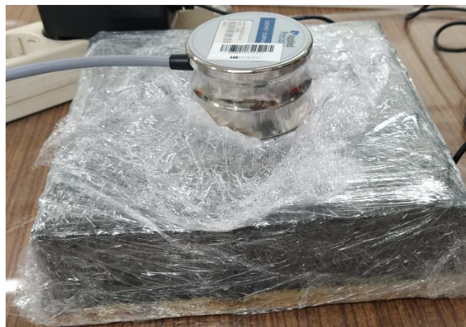
Figure 22: Thermal conductivity measurement of formulation 47 with ambient curing.
