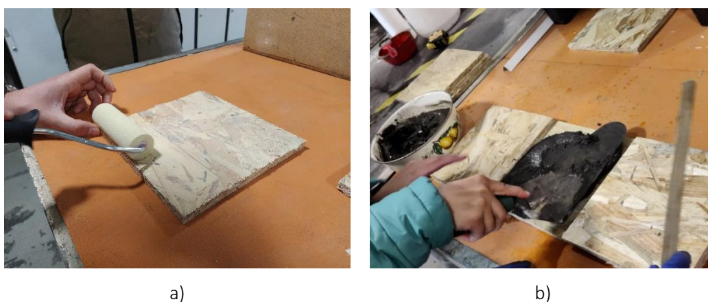
Figure 23: Application of the (a) primer and (b) waste-based render on the OSB board.
