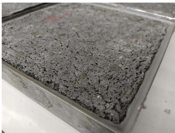
Figure 7: Metallic cup and specimen sealed with paraffin.
