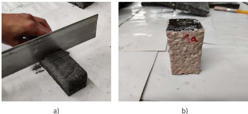
Figure 8: a) Cutting the specimens into two halves; b) Sealing the sides with epoxy resin.
