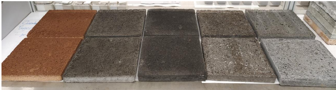
Figure 3: Example of the specimens for thermal conductivity measurement using the Guarded Hot Plate Method.
