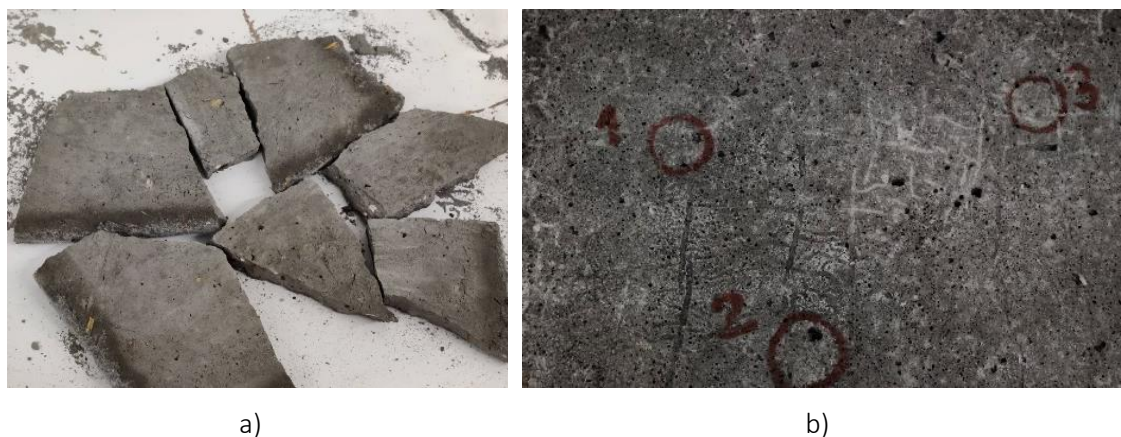
Figure 25: Hard body impact test results: (a) Waste-based render and (b) Cladding panel.
