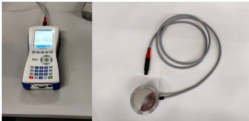
Figure 4: ISOMET 2114 – modified transient plane source equipment
