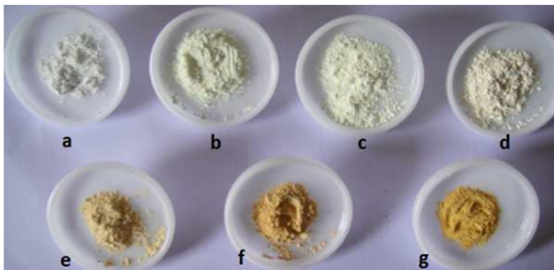
Figure 37 Photographs of Gd:Ce:Mo oxides prepared by a sol-gel method: a 1:1:0; b 1:0.95:0.05; c 1:0.9:0.1; d 1:0.85:0.15; e 1:0.8:0.20; f 1:0.75:0.25; g 1:0.65:0.35. Reproduced with
